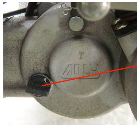
Gear oil level plug of differential
